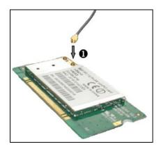
Insert the 802.11 card in the mini-PCI socket of the AX3000 circuit board. The 802.11 card must be first inclined at  $45^{\circ}$  then pushed horizontally **①**. The 802.11 card should automatically go to the horizontal position and locked by the two hooks **②**.
