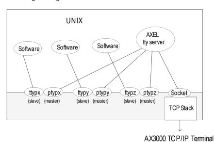
The following drawing shows the Unix/Linux mechanisms:
